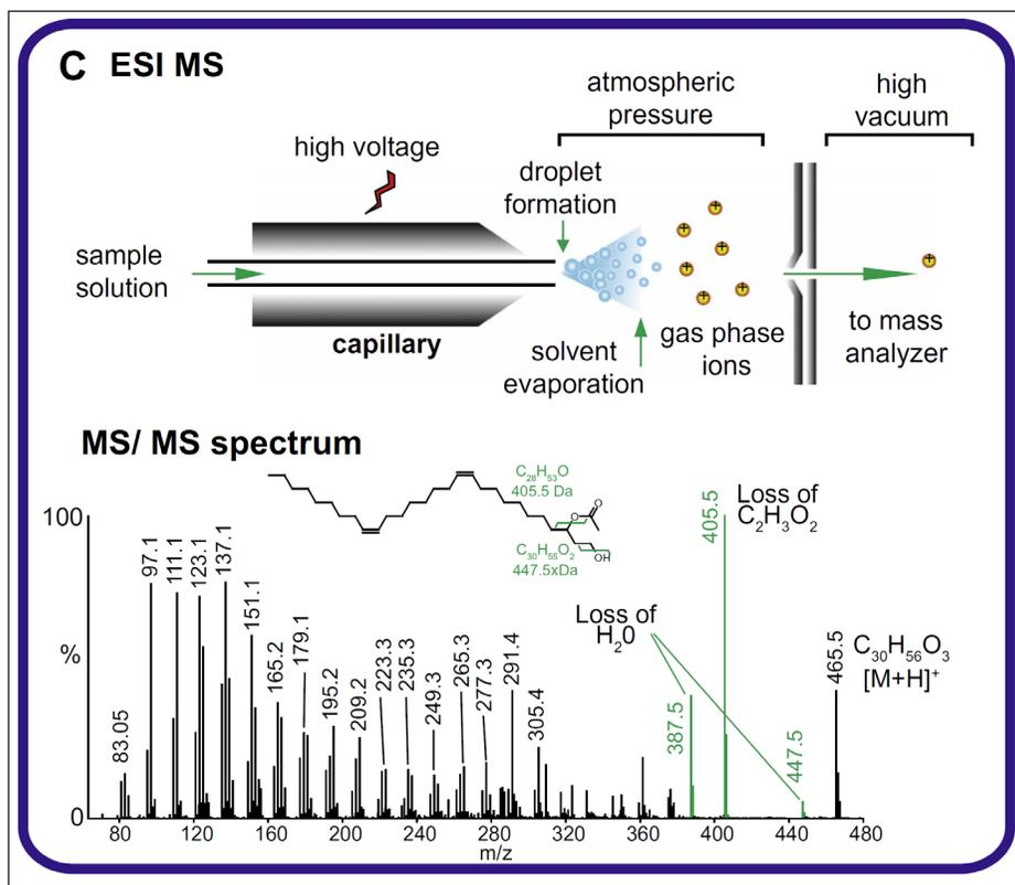
**Figure 4:** ESI-MS analysis, a sample dissolved in an organic solvent is introduced into a capillary. Applying a high voltage to the liquid generates a fine mist of droplets at atmospheric pressure. As the solvent evaporates and the droplets shrink, the analyte ions are released into the gas phase. The mass analyzer can select ions from a mixture based on their mass and subject them to fragmentation
