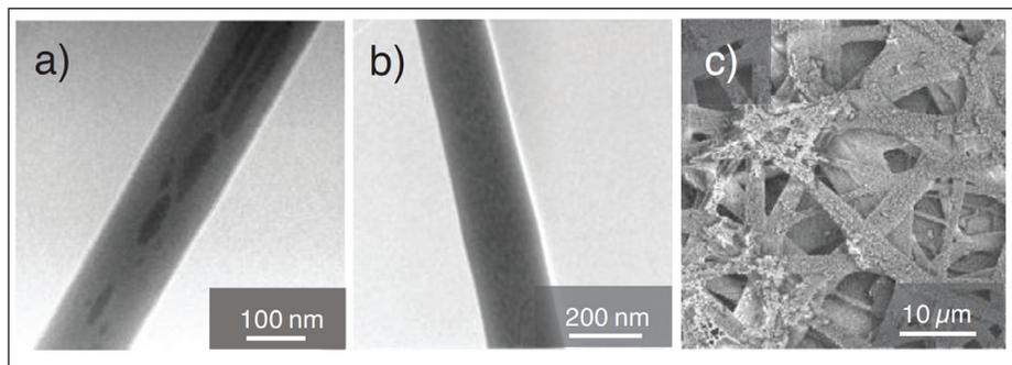
**Figure 20:** Pheromone-loaded fibers. TEM images of pheromone-loaded: (a) polyamide 6 (PA6); (b) cellulose acetate (CA) fibers after staining with ruthenium tetroxide; (c) Pheromone-loaded polyester fibers
