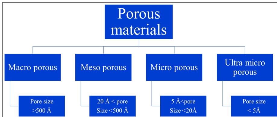
**Figure 21:** PTypes of pores based on pore size
