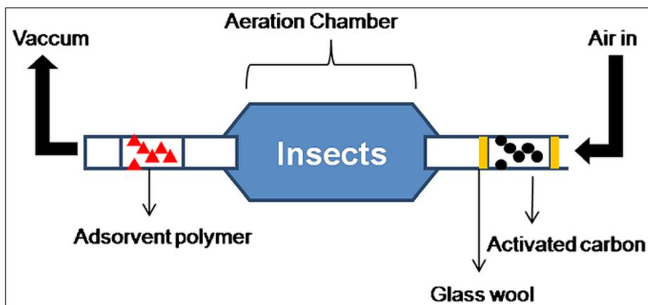
**Figure 1:** An aeration system used to collect insect volatiles for adsorption on a polymer
