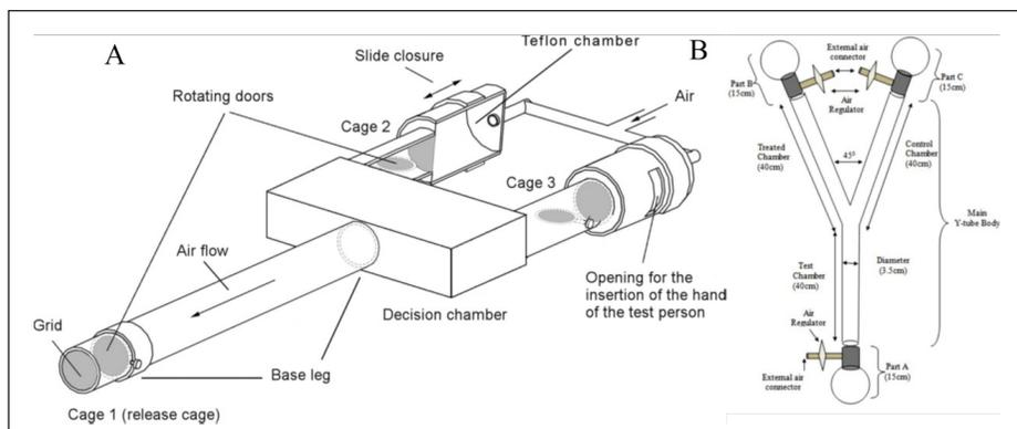
**Figure 13:** Configuration of olfactometer developed by Geier and Boeckh (1999) and Das (2021)
