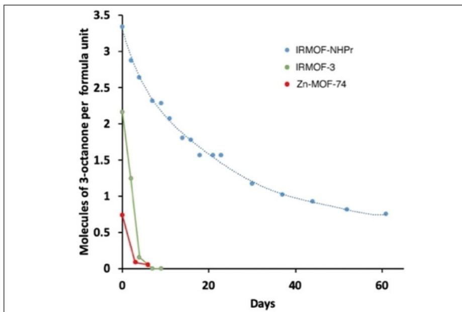
**Figure 24:** The amount of 3-octanone remaining in the loaded samples of IRMOF-3, IRMOF-NHPr and Zn-MOF-74 after more than 60 days of exposure to air was evaluated using  $^1\text{H}$  NMR spectroscopic analysis of the digested samples (Hamzah *et al.*, 2020)
