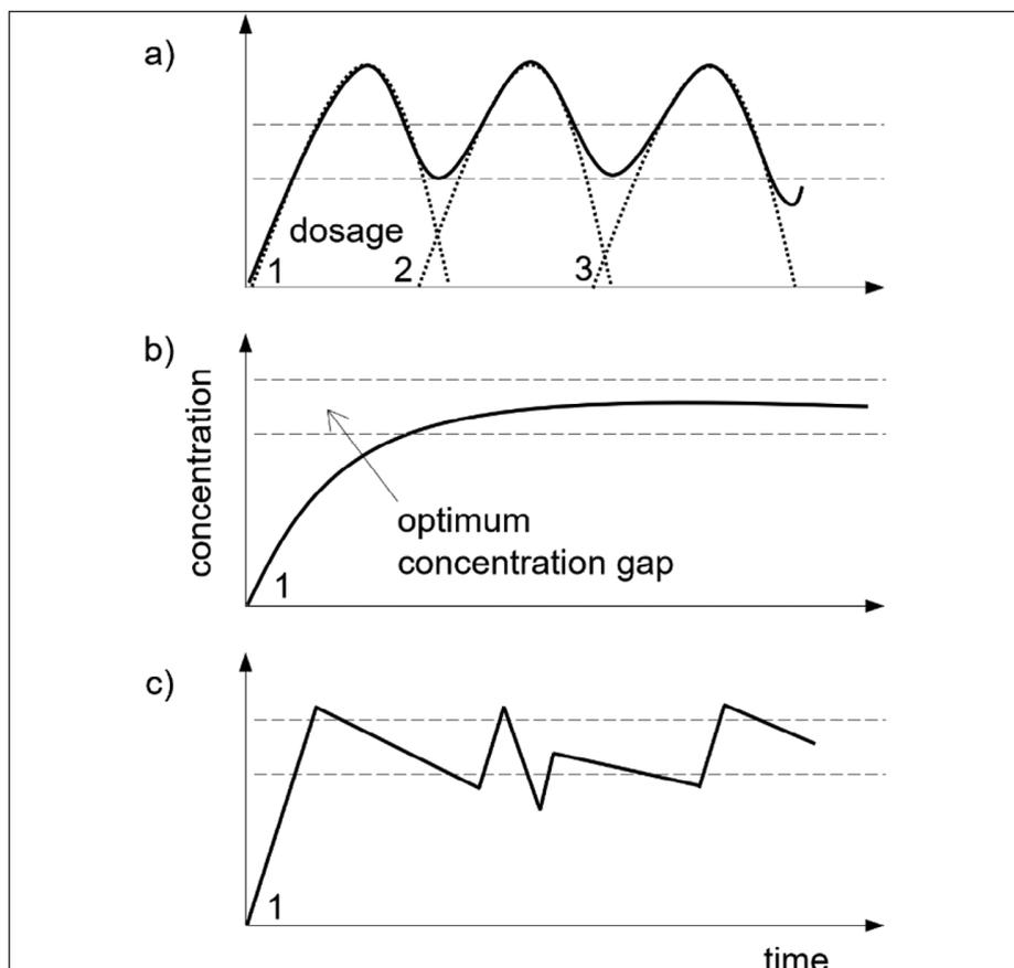
**Figure 17:** The concentration of pheromones over time depends on the release mechanisms used: a) Cumulative concentration resulting from the application of individual doses, b) Controlled release from a single dose over an extended period, c) Responsive release mechanisms, where varying release characteristics over time can be adjusted by activating the release of additional active substances through stimuli such as light, heat or magnetic pulses (Hellmann *et al.*, 2023)
