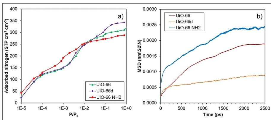
**Figure 23:** a) Nitrogen adsorption isotherm of MOFs at 77 K (with a logarithmic pressure scale) obtained through Monte Carlo simulations; b) Mean square displacement of 3-octanone within MOFs, calculated using molecular dynamics simulations (Doan, 2015)
