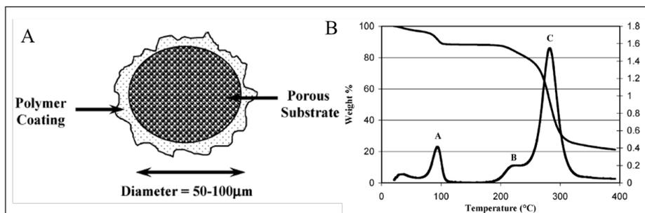
**Figure 24:** (A) Porous substrate coated with polymer. (B) Dynamic TGA analysis of dodecanol adsorbed onto MCC coated with a water-soluble polymer: (A) evaporation of dodecanol, (B) degradation of the coating and (C) pyrolysis of cellulose. The upper curve represents the actual weight loss thermogram, while the lower curve shows the first derivative of the thermogram with respect to temperature
