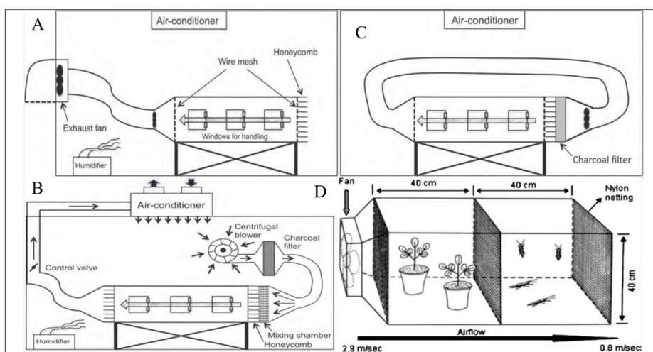
**Figure 12:** Various wind tunnel configurations are available for behavioral studies include: (A) pulling-air type wind tunnels, (B) pushing-air type wind tunnels designed for air recycling, (C) wind tunnels that combine both pushing and pulling air types and (D) setups where moths are exposed to odors from non-host pea plants within the wind tunnel (Zhang *et al.*, 2007; Kainoh, 2011)
