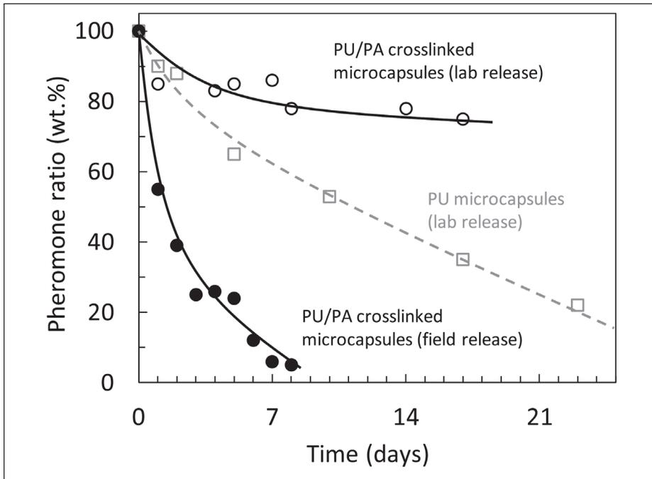
**Figure 15:** The release behavior of cross-linked microparticles made from polyurethane (PU) and polyurethane/polyamide (PU/PA) was studied under both laboratory and field conditions (Hellmann *et al.*, 2011)
