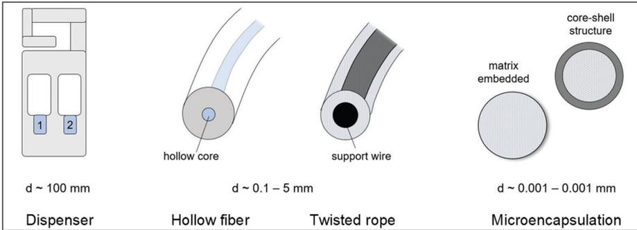
**Figure 14:** Pheromone release systems (pheromone indicated in light blue,  $d$  = diameter)
