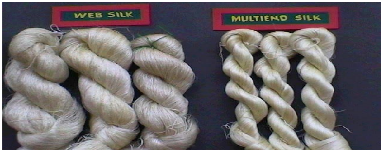
Fig. 3. Photograph showing the comparison between web structured bulky raw silk and heavy denier silk reeled from same number of cocoons
