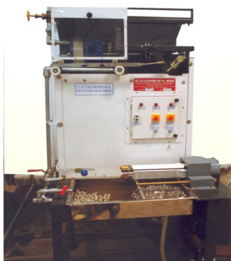
Fig. 2. The proto type model bulky raw silk reeling machine developed by CSTR
