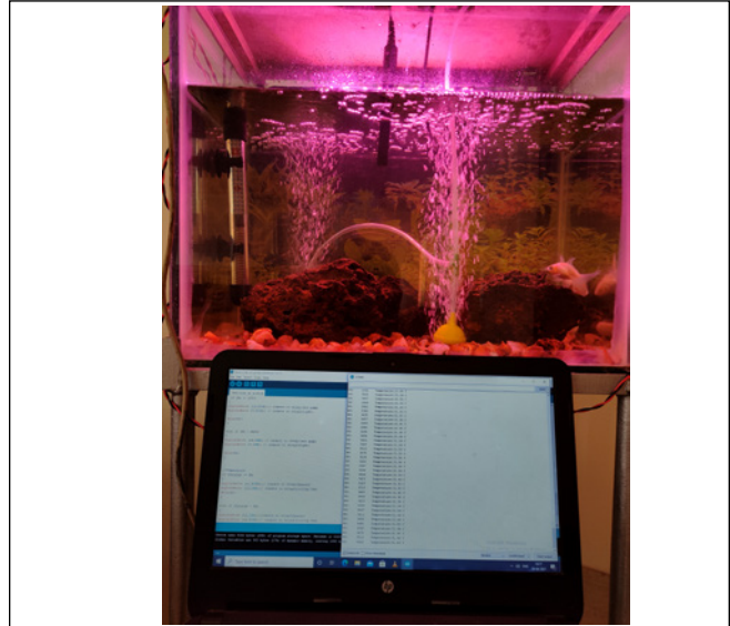
Figure 6: Light & DO control through Arduino
