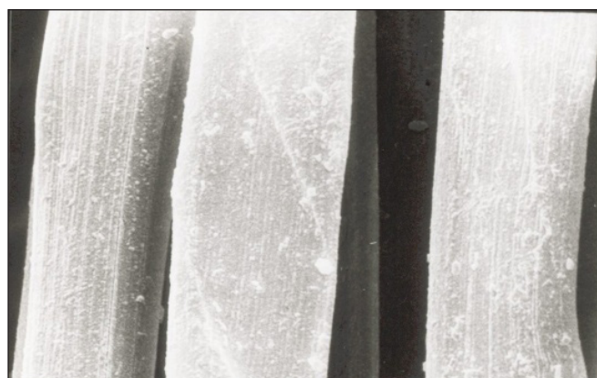
Figure 1: Scanning electron photomicrograph of single silk filaments reeled from oak tasar ( Antheraea proylei J. ) cocoons. The cocoons were cooked prior to reeling by a standardized pineapple extract procedure involving initial 30 min pressure cooking followed by 12 hr soaking in pineapple extract at room temperature (26-31 °C)
