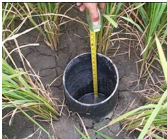
Figure 4: Irrigation scheduling when the water depths below 15 cm
