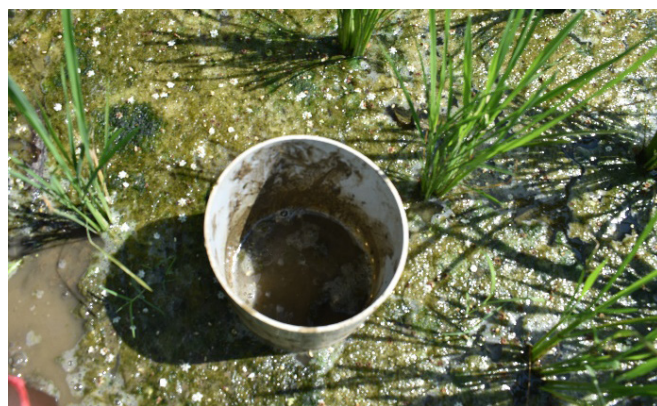
Figure 2: A field tube in flooded field
