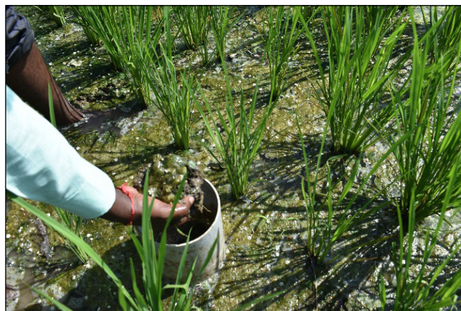
Figure 3: Removal of the soil inside PVC pipe
