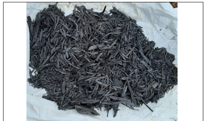
Figure 1: Biochar prepared using sugarcane bagasse
