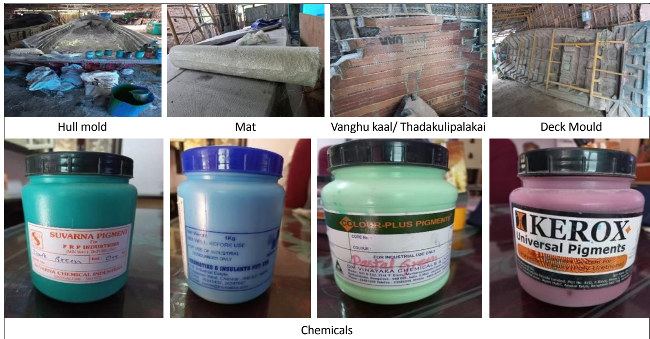
Figure 2: Materials used for making of FRP Boat
