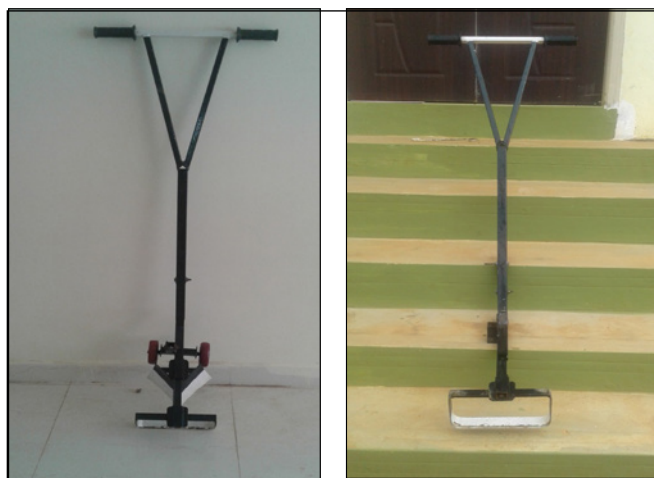
Figure 1: Groundnut weeder cum earthing-up tool before and after modification
