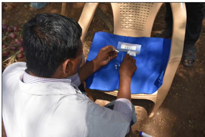
Figure 2: Examination SCC using Tanucheck SCC kit
