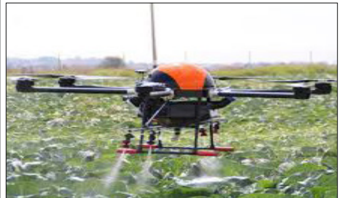
Figure 2: Drones Easy-to- fly devices that are designed to spray pesticides on crops. It is possible to capture high resolution images of whole field for further analysis
