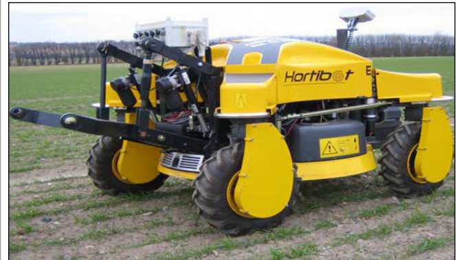
Figure 1: Hortibot It is about 3-foot-by-3foot. is self-propelled. and use global positioning system (GPS). It can recognize 25 different kinds of weeds and eliminate them by using its weed-removing attachments.
