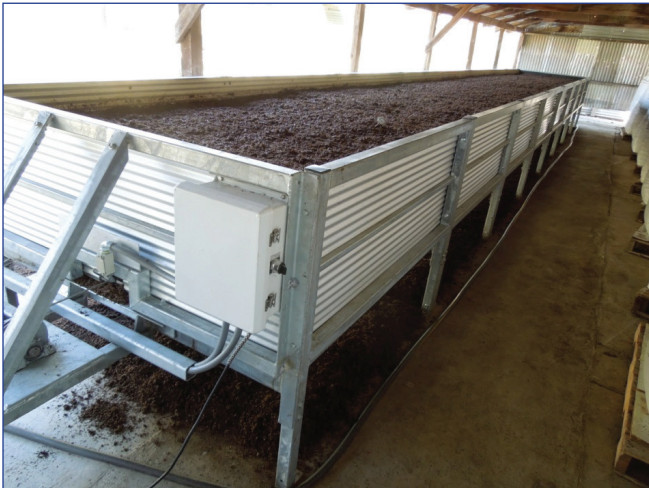
Figure 1: Large scale vermicomposting (continuous flow)
