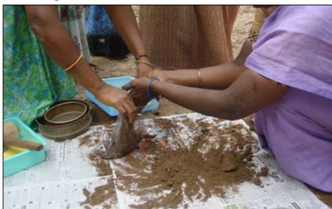
Figure 12: Collect the sample in a clean polythene bag
