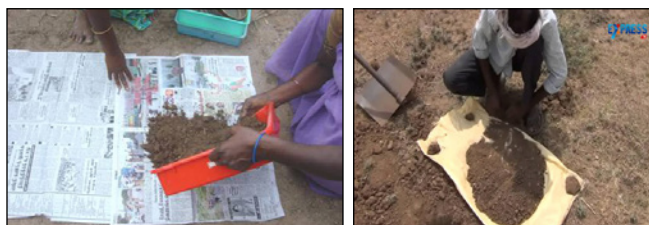
Figure 8: Mix the soil samples thoroughly
