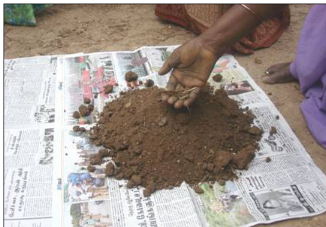
Figure 9: Remove foreign materials like roots, stones, pebbles and gravels
