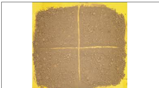
Figure 10: Quartering is done by dividing the thoroughly mixed sample into four equal parts
