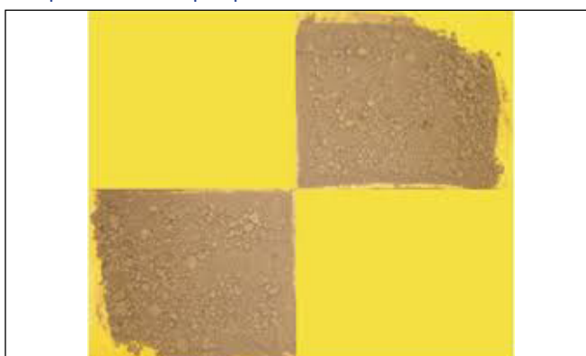
Figure 11: Two opposite quarters are discarded and the remaining is mixed
