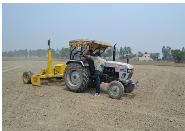
Fig. 3. Land levelling with laser land leveller for DSR
