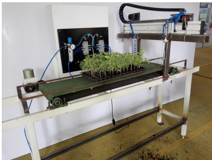
Fig. 2. Development of a robotic pick-up and transplanting unit
