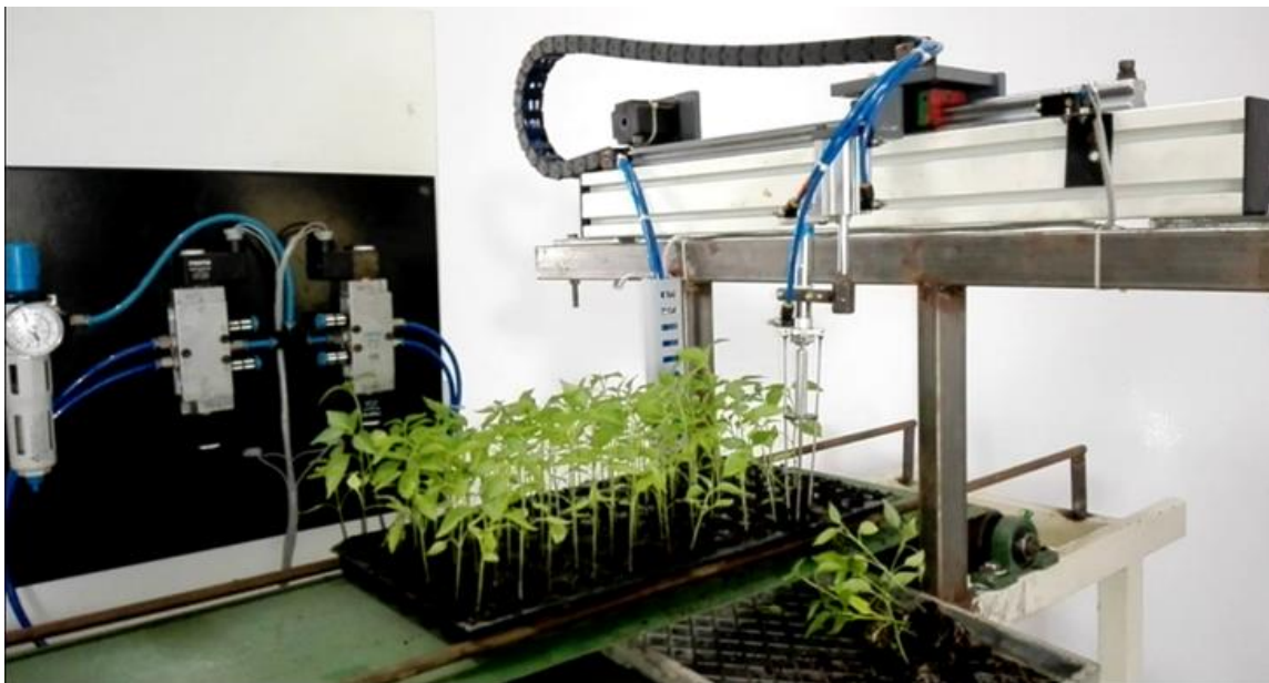
Fig. 4. Performance evaluation of robotic pickup and transplanting system for protray grown vegetable seedlings
