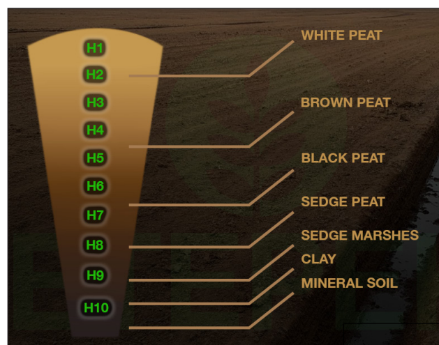
Figure 3: Raw sphagnum peat moss is graded using the Von Post scale (Lopez, 2017)
